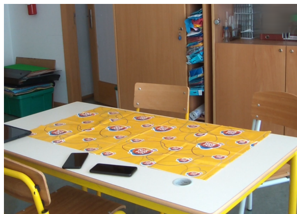
Figure 4.1: Patterned paper placed on top of a surface to facilitate plane detection.
